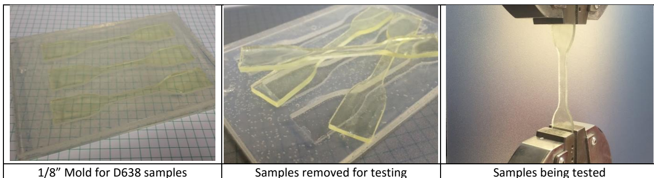
Figure 2. ASTM D638 Tensile Properties of Plastics, sample preparation and test fixture.
